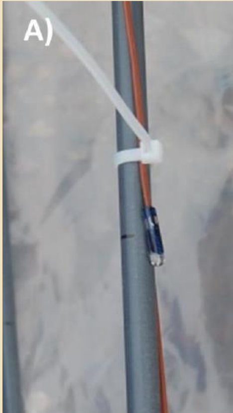
Thermocouple on temperature monitoring "stick."
